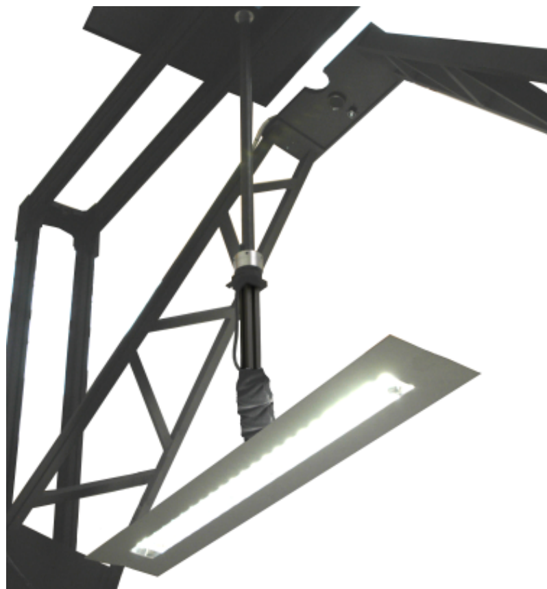
Figure 4.1.: Ceiling light (for office lighting, for example) in near-field goniometer
