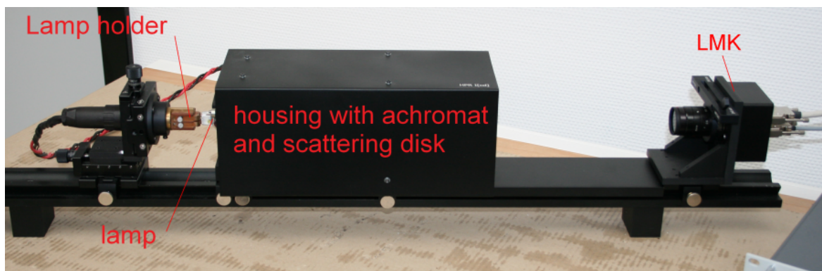
Figure 4.5.: CMS measuring equipment for adjustment of cold light reflector lamps
