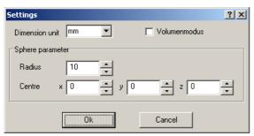
Using this dialog (dialog section "SPHERE PARAMETER") the position and the radius of a sphere can be fixed. The unit of measurement for the indications of size and orientation of the following dialog sections can be modified via the combined box "Dimension unit". If the selection box "VOLUME MODE" is activated, then the starting points of those rays which
