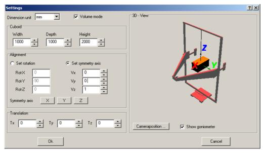
Using this dialog, the position and the side lengths of a cuboid can be fixed. "WIDTH" is the side length in the direction of Y, "DEPTH" is the length in the direction of X, and "HEIGHT" is the length in the direction of Z.
