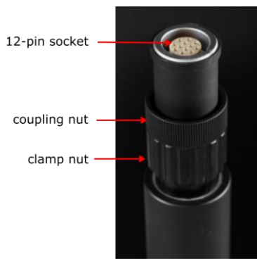
Figure 9: Plug interface
