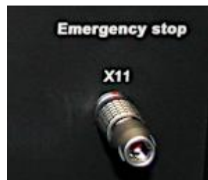
Figure 15: Emergency-stop circuit connector at the back panel
