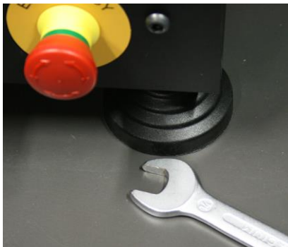
Figure 17: open-end wrench for turning the mounting feet
