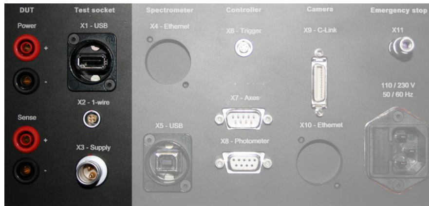
Figure 11: Back panel connections to DUT mount plug interface
