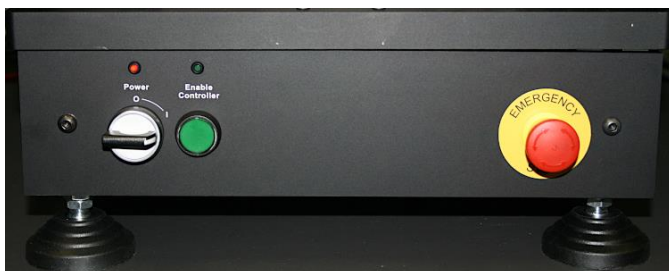
Figure 14: Emergency-stop switch at front panel
