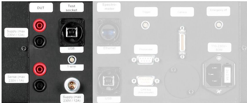
Figure 10: Back panel connections to LED mount plug
