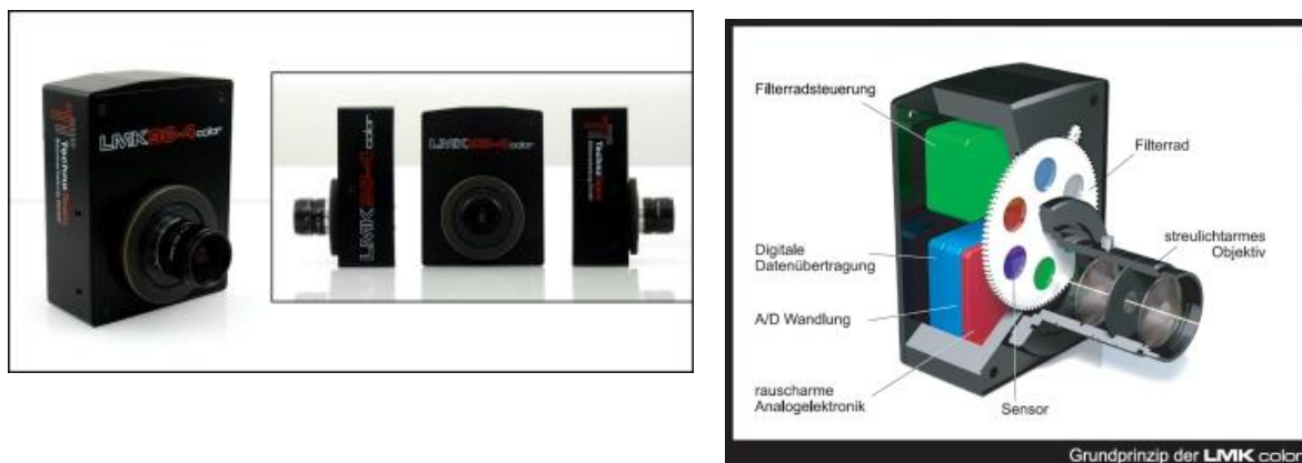
Figure 5: LMK98 with filter wheel
